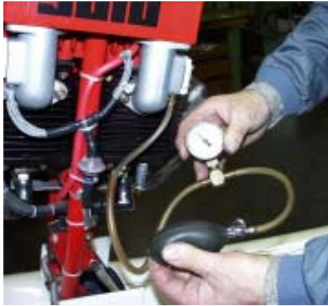
Picture 7: Test of air-tightness
