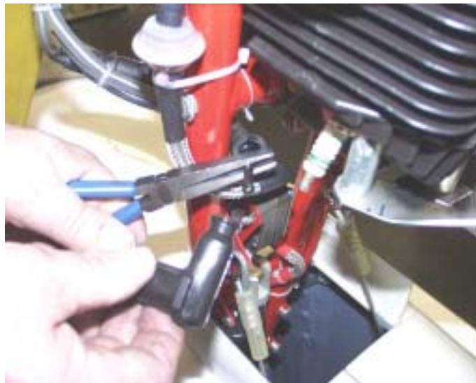
Picture 9: Replacement of spark-plug connector
