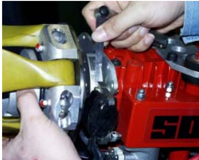
Picture 11: Examination of distance of ignition coils
